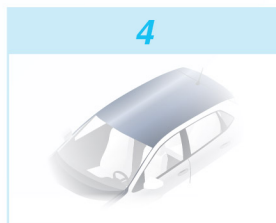
4 ROOF LINERS RIGID FOAM
